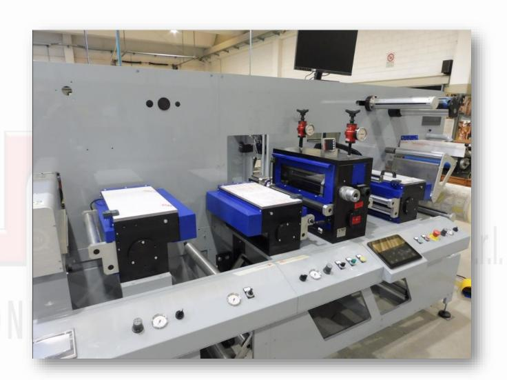
> EASYLINER WASTE-REMOVING REWINDING UNIT:
