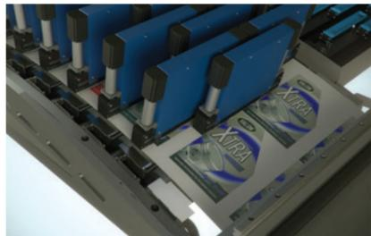
Micro-motor controller technology ensures that all heads are positioned precisely, calibrated to print as one, enabling seamless print across the full web width.
