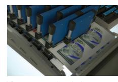
Micro-motor controller technology ensures that all heads are positioned precisely, calibrated to print as one, enabling seamless print across the full web width.
