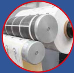
**Contact matrix stripping option** for high speed stripping of difficult label shapes
