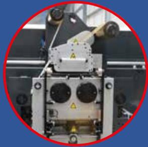
**Flat bed hot foiling station** with foil saver
