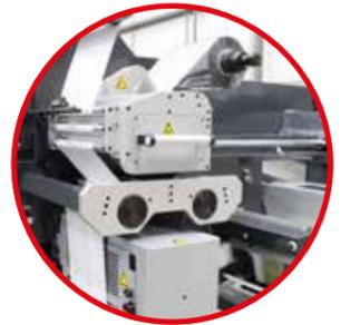
**Semi rotary hot foil station** with foil saver
