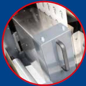
**Hot air dryer option** for aqueous varnishes and coatings
