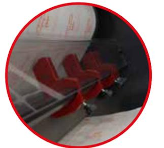
**Scissor, Razor and Crush slitting modules** with 5 holders
