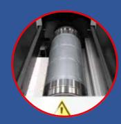
Full rotary die cut option. Enables the use of rotary dies from 12" (305mm) to 25½" (648mm).
