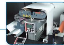
**Web guide sensor - edge sensor, Line camera(Optional)**
