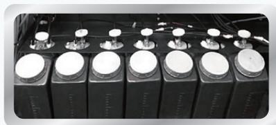
Double-inlet bulk tank with a liquid level sensor is easily used for adding ink and alarming for the shortage of ink.
