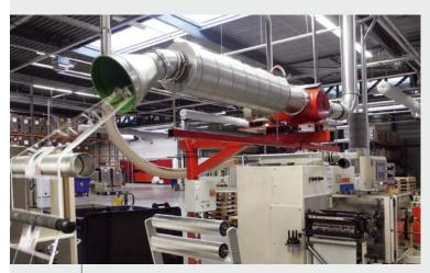
Application: Cutting system for self-adhesive matrix and trims
