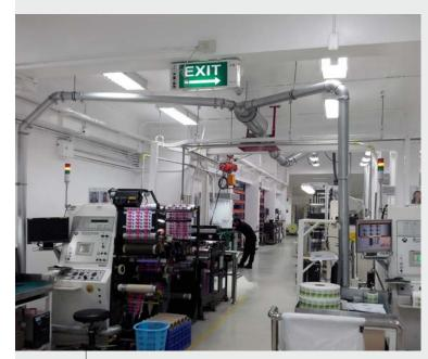
Application: TCM-160 installed below the roof for four edge trims from two label slitters
