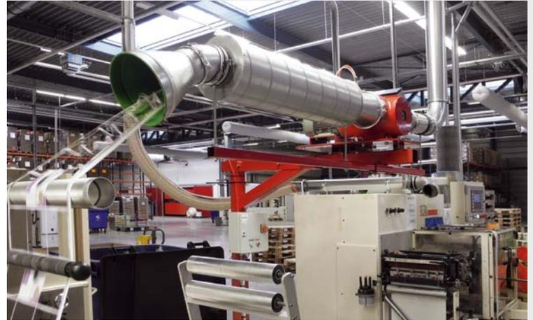
**Application:** Cutting system for self-adhesive matrix and trims
