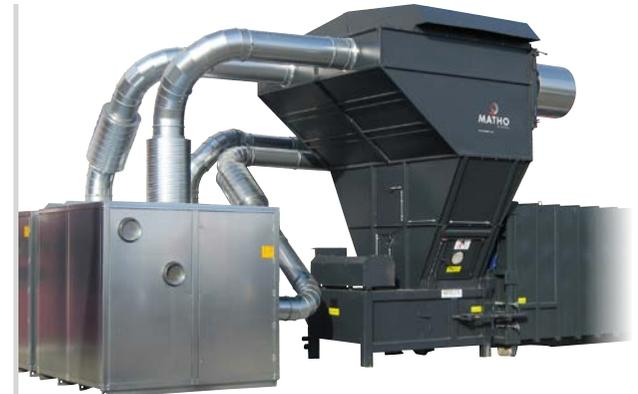
Our central systems are dedicated to extract and cut the waste of plenty of production machines centralized from the complete production site. There are a lot of different disposal solutions available, either new ones or already existing ones (baler, static compactors, portable compactors, screw compactors, etc.).
