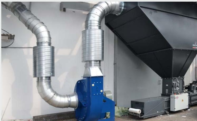
Application: Large matrix removal system for ten machines including a baler
