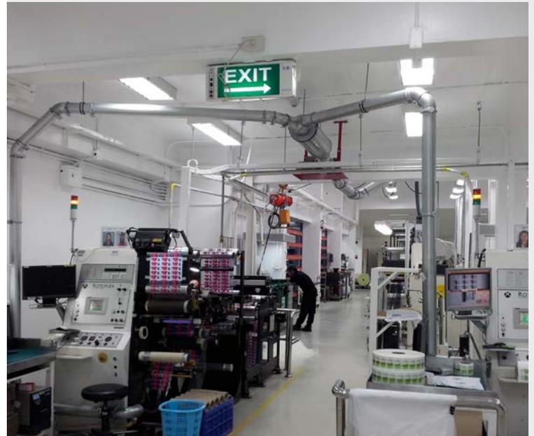
**Application:** TCM-160 installed below the roof for four edge trims from two label slitters
