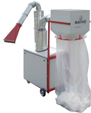
Local and stand alone systems into PE-bags, Big Bags or Screw compactors. Every system is equipped with a machine frame, transportation fan, material separator, cutting unit and electrical control box.
