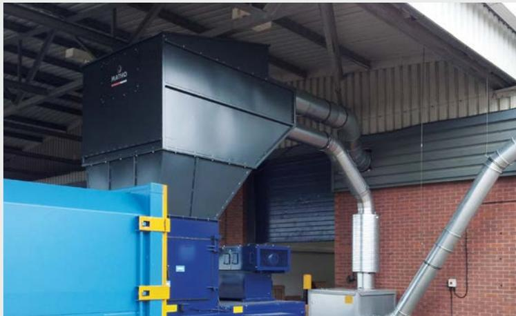
Application: Matrix removal system into a static compactor including an air return system and a sound enclosure for the transportation fan
